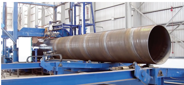
Spiralweld pipe is formed and welded from long rolls of steel.
