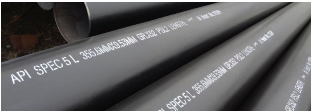
Pipe steel for transmission pipelines must be certified as meeting quality standards and requirements.
