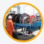
A "smart pig" being readied for an internal pipeline inspection
