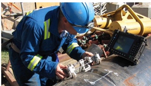
A technician scans pipe with ultrasonic imaging technology
